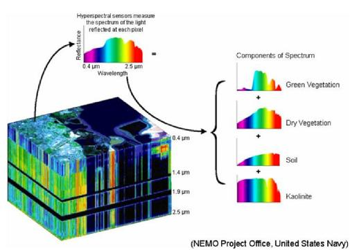
Figure C8-1: Hyperspectral data "cube" with examples of some spectral profiles
